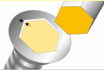
• Screwdriver bit with external hexagon profile.
